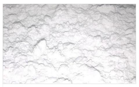
**MMS GYP FLOUR** is a high quality Gypsum product ground to mean average particle size of 18 microns.
